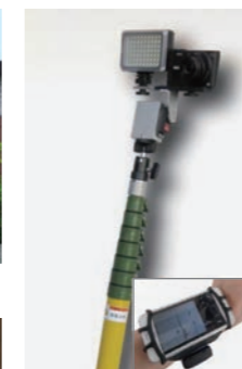
Conducting an inspection using a robotic camera designed for attic inspection
