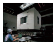
Full-sized exterior walls are tested for anti-seismic performance
