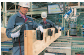
Metal fittings are pre-attached to structural frames to reduce the workload at construction sites
